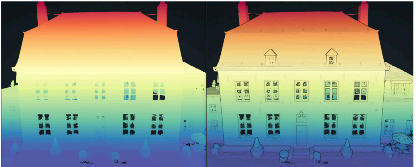
Same point cloud without EDL (left) and with it (right), Radius and Strenght parameters impact the degree of edge shadowing @ULB
